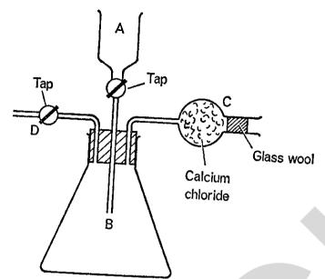
A known mass of the carbonate is placed in flask B, dilute hydrochloric acid is placed in funnel A and the whole apparatus is weighed. The acid is then added to the carbonate and when the reaction is over, air is blown through tube Dand the whole apparatus re-weighed.
