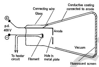
The diagram shows a section through an apparatus for producing an electron beam from a heated filament to a fluorescent screen.
