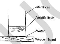
A metal can containing a volatile liquid, such as ether, stands on a wooden board with a layer of water between its base and the board. When a jet of air is blown through the liquid, the water freezes. Explain why this happens. (4)
