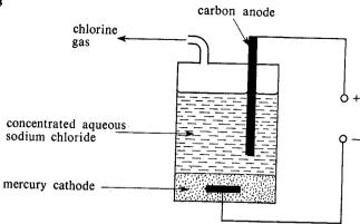
When concentrated aqueous sodium chloride was electrolysed using the above apparatus, chlorine gas was given off at the anode. At the cathode no gas was given off, but sodium ions were discharged, setting free sodium, which dissolved in the mercury to form sodium amalgam. Sodium amalgam (a mixture) can be represented by the formula Na/Hg. When sodium amalgam was added to water, hydrogen gas, sodium hydroxide and mercury were formed.
