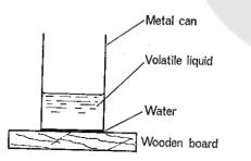
A metal can containing a volatile liquid, such as ether, stands on a wooden board with a layer of water between its base and the board. When a jet of air is blown through the liquid, the water freezes. Explain why this happens. (4)
