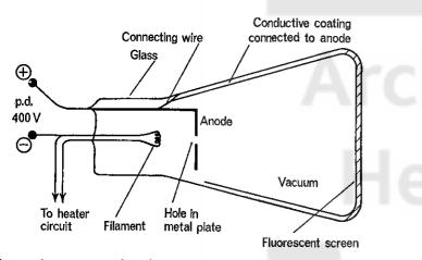
The diagram shows a section through an apparatus for producing an electron beam from a heated filament to a fluorescent screen.
