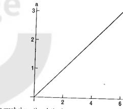
The above graph shows the relation between a, the current in amperes, and v, the potential difference in volts, for a fixed resistor. What is the resistance of the resistor?
