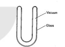
The diagram illustrates a double-walled vacuum flask used for keeping its contents hot. (a) Why is a vacuum required between the two walls?
