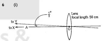
Rays of light from a point X on the edge of the sun's disc are effectively parallel. The lens in the diagram, which has a focal length of 50 cm, is arranged so that its principal axis OA points towards X. Where will the rays from X come to a focus after passing through the lens? [2]
