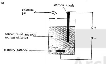
When concentrated aqueous sodium chloride was electrolysed using the above apparatus, chlorine gas was given off at the anode. At the cathode no gas was given off, but sodium ions were discharged, setting free sodium, which dissolved in the mercury to form sodium amalgam. Sodium amalgam (a mixture) can be represented by the formula Na/Hg. When sodium amalgam was added to water, hydrogen gas, sodium hydroxide and mercury were formed.
